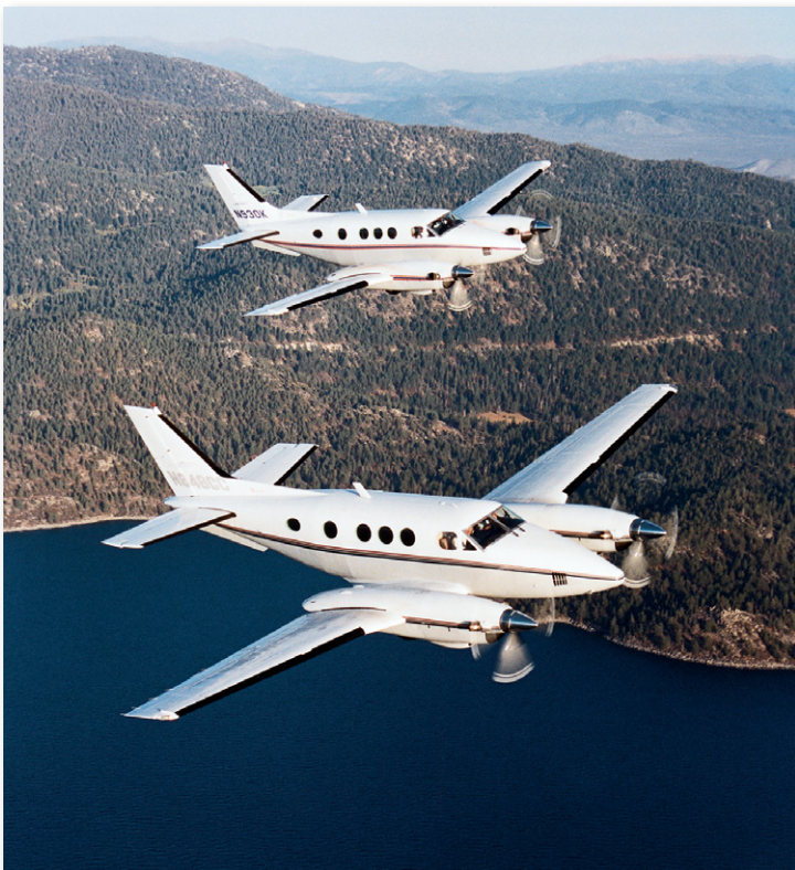
At left, an E90 (foreground) flies in close formation with an A90 over Lake Tahoe in Northern California. Both are equipped with Raisbeck's 4-Blade Power Props, Dual Aft Body Strakes, Gross Weight Increase and Wing Lockers.
