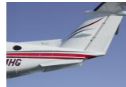
Dual Aft Body Strakes have a positive effect on yaw dampening
