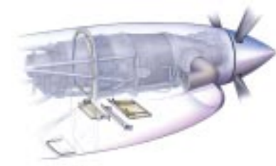
Raisbeck RARS provide a cooler engine, more horsepower, and fuel savings
