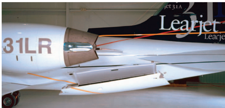
Raisbeck offers its ZR Lite modification for the Learjet 31, top, and the Learjet 35/36. The mod increases range of the Learjet 31 by 5 to 11 percent. On the 35/36 model, Raisbeck uses a "batwing," right, behind the trailing edges to increase range by 6 percent. The aft fuselage locker, above, has a maximum capacity of 300 pounds to give passengers more room to store their belongings.
