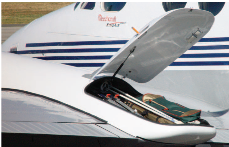
Raisbeck's modifications to the King Air allow operators to squeeze as much performance as possible out of the turboprops. Clockwise: the ram-air recovery system is designed to deliver improved climb performance, while the quiet turbofan propellers provide a "virtually vibration-free operation." The Crown wing lockers provide 17 cu ft of additional stowage space.
