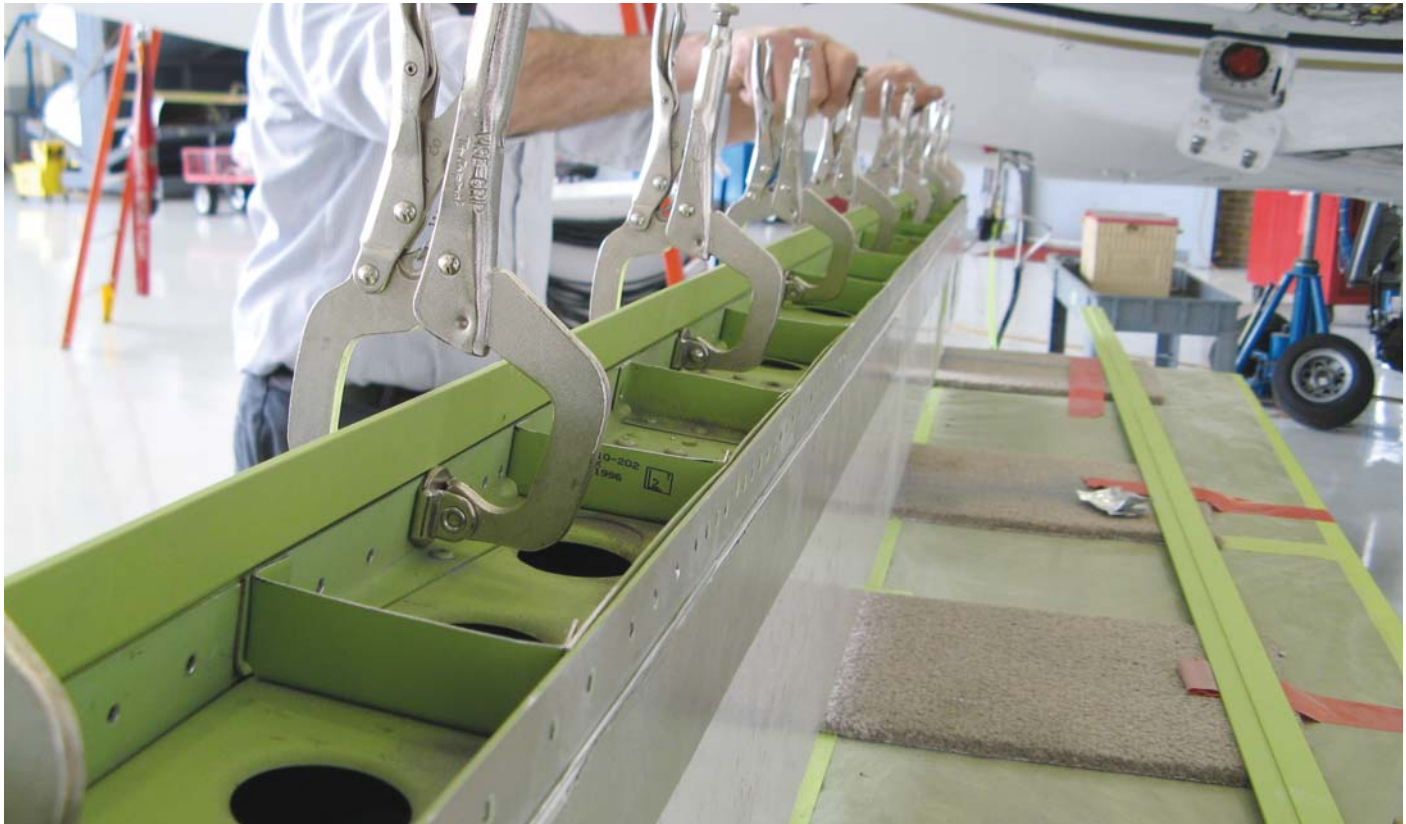
PART OF RAISBECK'S ZR LITE PROCESS: A 'ZEE' IS BEING INSTALLED ONTO THE EXISTING PORTION OF FLAP, AFTER WHICH RAISBECK INSTALLS ITS NEW COMPOSITE FLAP ONTO THE ZEE.
