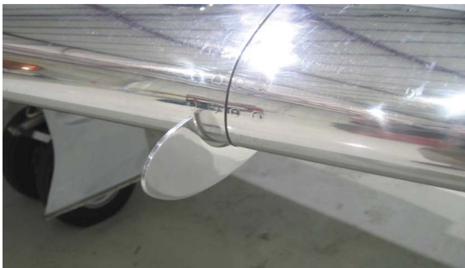
A WING VORTILON (FOUR TOTAL (TWO PER WING)) PLACED BY RAISBECK ON THE LEADING EDGE OF THE WING TO IMPROVE LOW SPEED PERFORMANCE, AND IMPROVE AIRFLOW EFFECTIVENESS.
