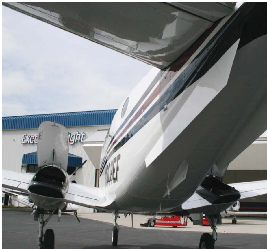
DUAL AFT BODY STRAKES IMPROVE THE STABILITY AND CONTROL, AND REDUCE DRAG IN ALL FLIGHT MODES ON ALL KING AIR MODELS.
