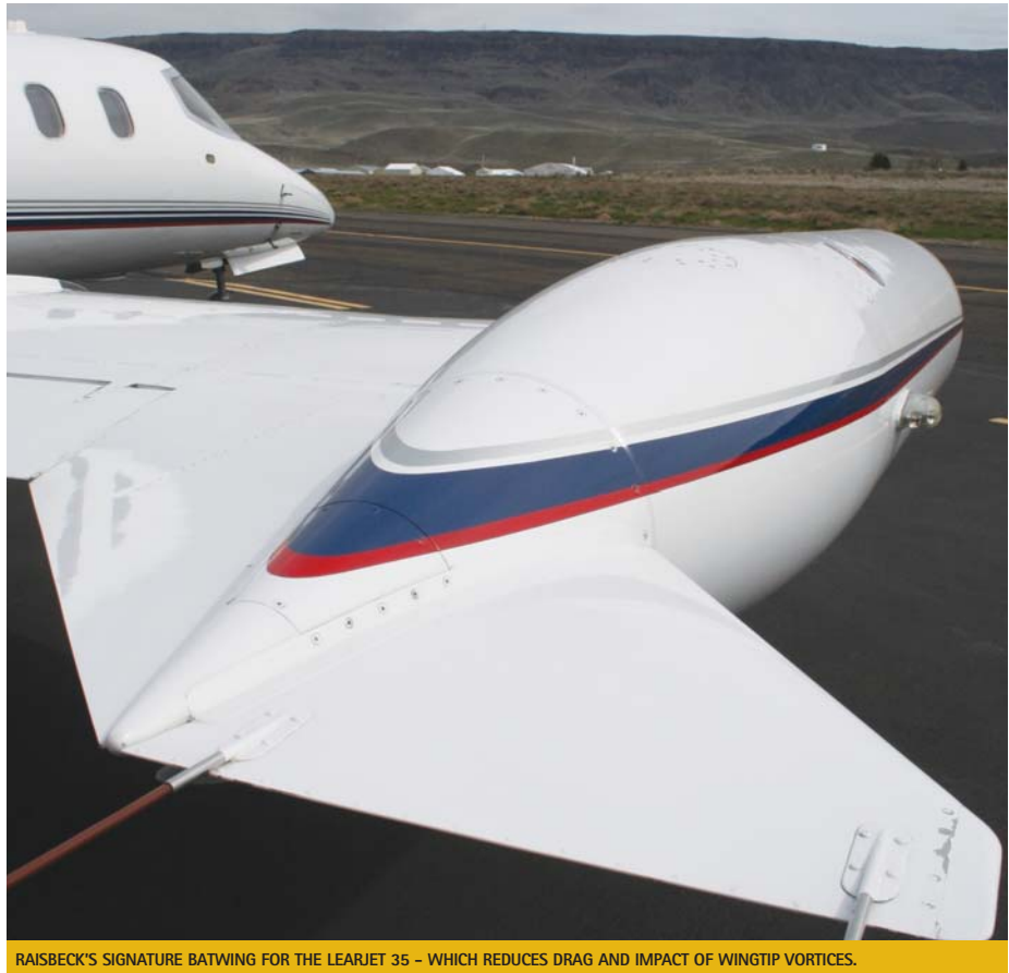
RAISBECK'S SIGNATURE BATWING FOR THE LEARJET 35 – WHICH REDUCES DRAG AND IMPACT OF WINGTIP VORTICES.
