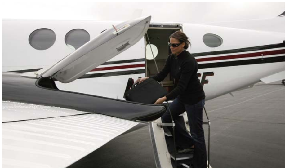
RAISBECK'S CROWN WING LOCKERS, AVAILABLE FOR ALL KING AIR C90S (INCLUDING C90GT, C90GTI), ALL 200S (INCLUDING B200GT) AND 300/350 (STANDARD ON THE 350 PRODUCTION LINE), OFFER CONVENIENT BAGGAGE/EQUIPMENT SPACE OUTSIDE OF THE CABIN.
