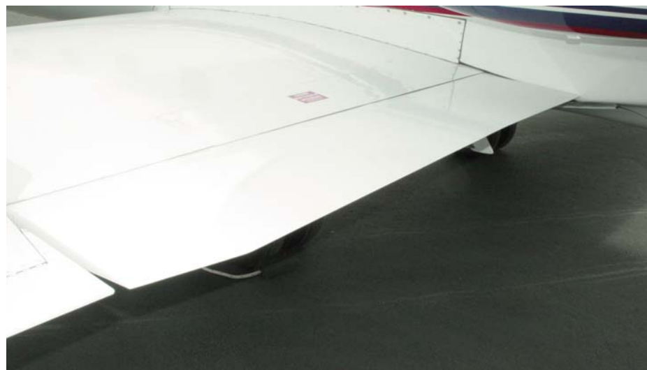
EXTENDED FLAPS REDUCE HIGH SPEED DRAG AND IMPROVE LIFT DISTRIBUTION (ON BOTH THE LEAR 35 AND LEAR 31).
