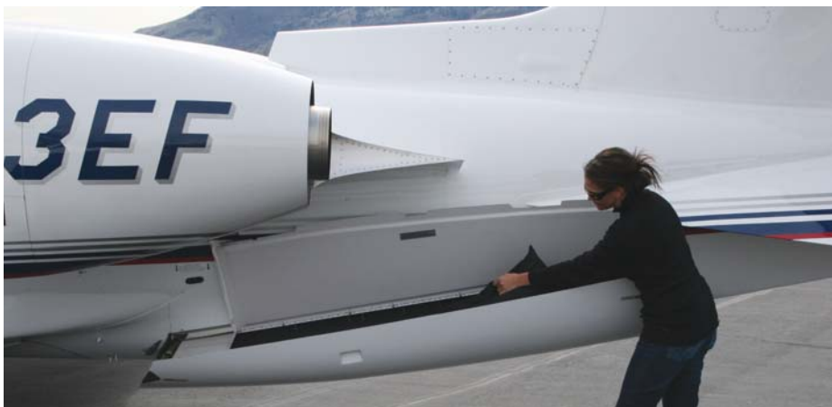
AN AFT FUSELAGE LOCKER ALLOWS FOR 300LBS OF STORAGE OUTSIDE OF THE CABIN AND MOVES THE CENTER OF GRAVITY FARTHER AFT ALONG THE AIRCRAFT, RESULTING IN LESS NOSE-UP TRIM AND REDUCING DRAG. THIS MOD IS AVAILABLE FOR BOTH THE LEARJET 35 AND 31 MODELS.
